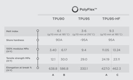
A Column: Extrusion multiplier 100% B Column: Extrusion multiplier 120% C Column: Extrusion multiplier 115%
