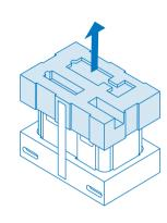
2 Cut the tape, remove the top foam, and unpack accessories.
