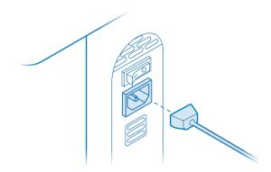
7 Connect the power cable to the machine and an outlet.
