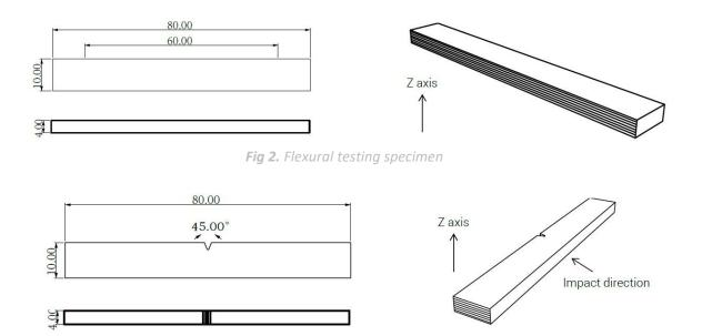
Fig 3. Impact testing specimen
