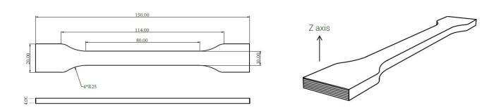
Fig 1. Tensile testing specimen
