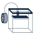
3 Heat up the extruder temperture to **210°C**, recalibrate your printing platform and start printing. To remove the finished part without destruction, the printer bed has to be heated to about **110°C**.
