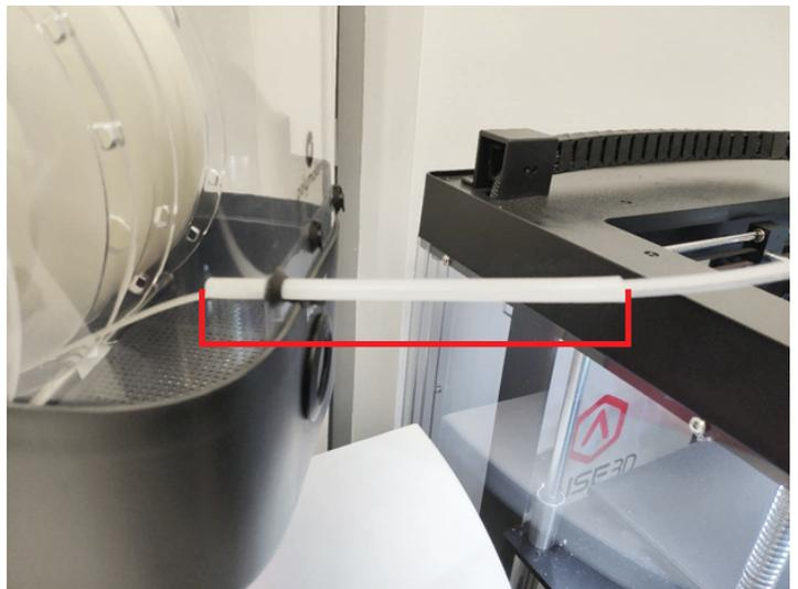
Disconnect the right hot end's feed tube from the blue coupler located on the right side of the machine. Press and hold the blue ring on the coupler to release and slowly remove the tube
