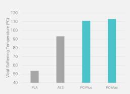
\*Tests performed with 3D printed specimens (100% infill, standard Vicat conditions)
