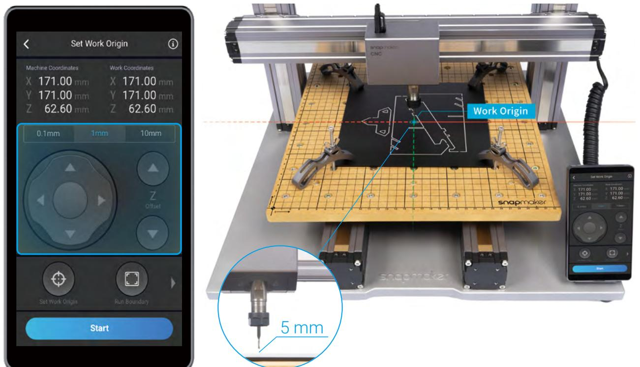
3. Place the Calibration Card or a piece of A4 paper between the CNC Bit and the material. Keep adjusting the height of the CNC Bit using **Z-** or **Z+** buttons until you feel slight resistance when you pull out the Calibration Card, and it should be wrinkled when you push it forward. Tap **Set Work Origin**.
