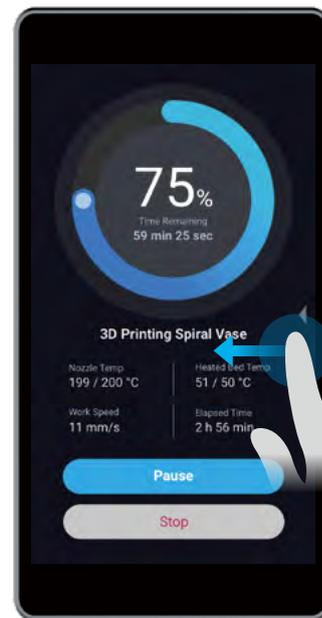
If poor adhesion occurs, swipe left on the printing progress screen and try adjusting the Z Offset. Or you can try leveling the Heated Bed again by selecting **Calibration**. Make sure the tip of the nozzle is clean before you calibrate the bed.
