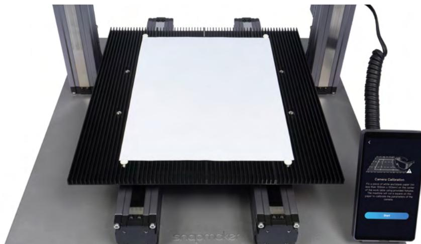
2. Tap **Start**, and the machine will use the engraved square to calibrate the camera.
