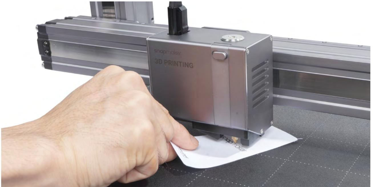
3. Keep adjusting the height of the nozzle using **Up** and **Down** buttons, until you feel slight resistance when you pull out the Calibration Card, and it should be wrinkled when you push it forward. Tap **Save** to save the calibration settings.
