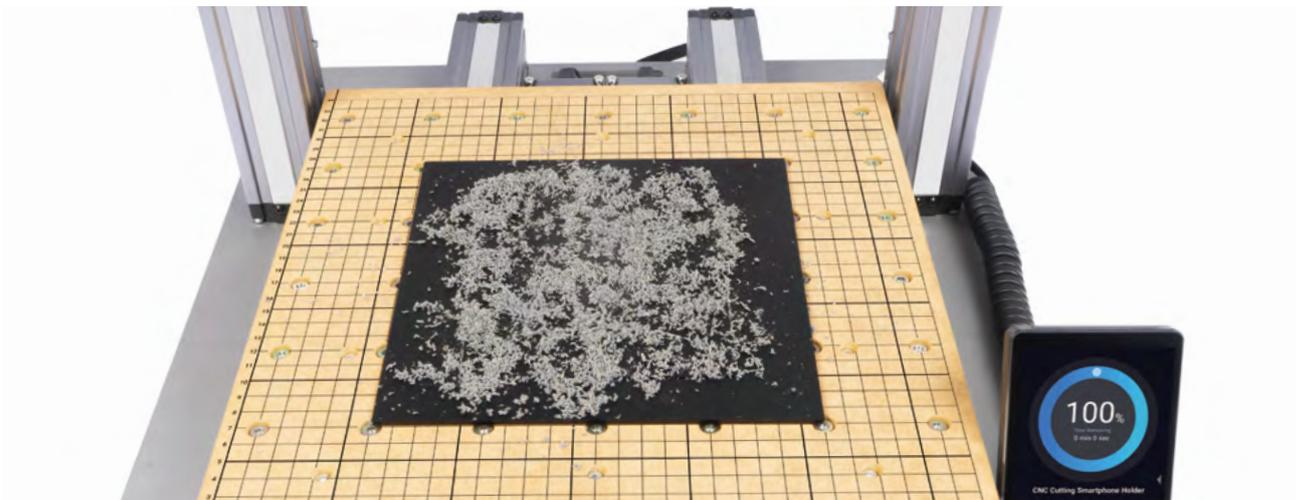
2. Clean the finished work and the machine with a dust collector, and then remove the finished work using the diagonal pliers.
