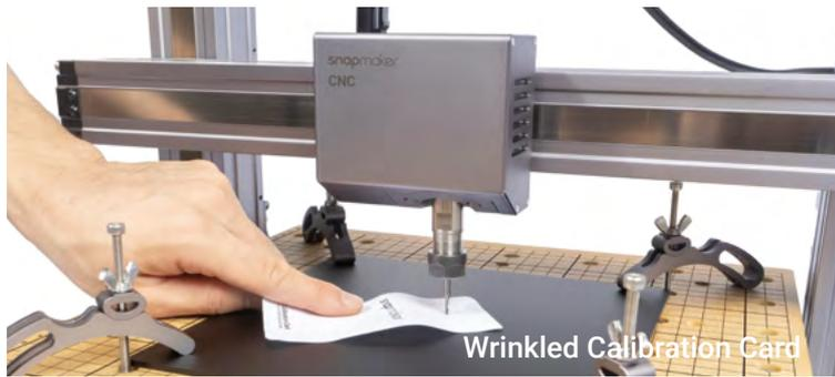
4. Tap **Z+** to lift the CNC Bit until it is above the clamp set, and then tap **Run Boundary** to check if the Work Origin is proper. If any part of the boundary trailed by the CNC Bit goes outside of the material, or if the CNC Bit runs into any portions of the machine, reset the Work Origin and run boundary again.
