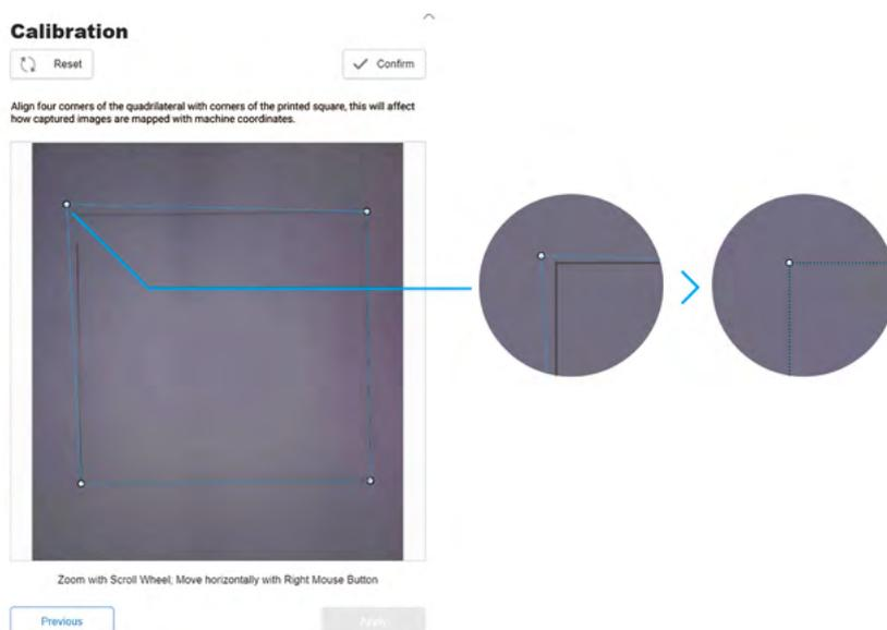
Click **Confirm** and the finished image will be loaded into the quadrant in the coordinate system. You can repeat the steps above if the edges of the captured image are still not aligned.
