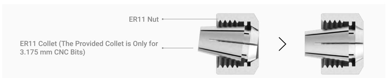
2. Put on the CNC Safety Goggles. Insert the CNC Bit into the ER11 collet (Flat End Mill is required for our provided model). Keep pushing the CNC Bit until its end bottoms against the shell of the ER11 collet.
