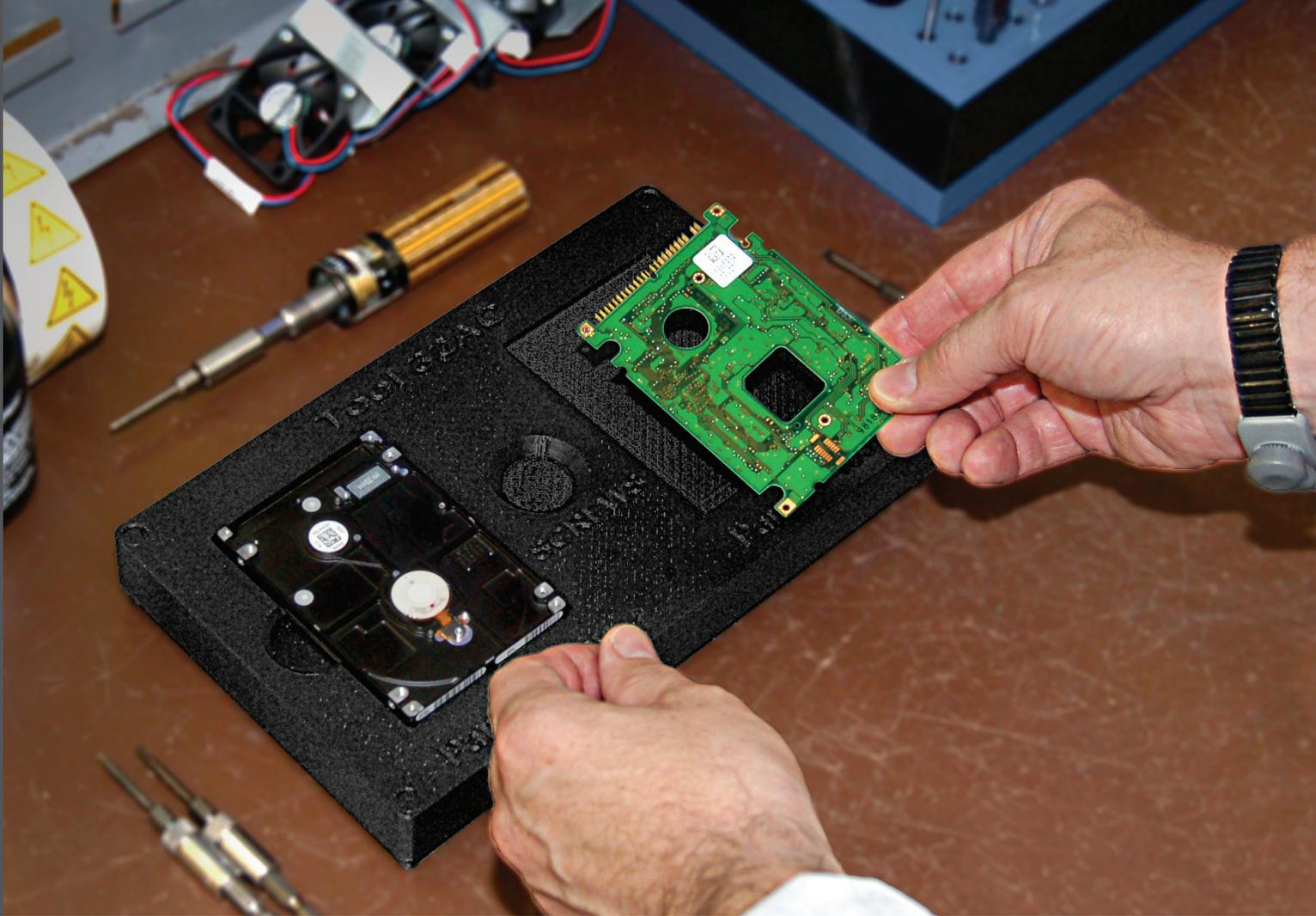
An assembly fixture for electronics made from ABS-ESD7.
