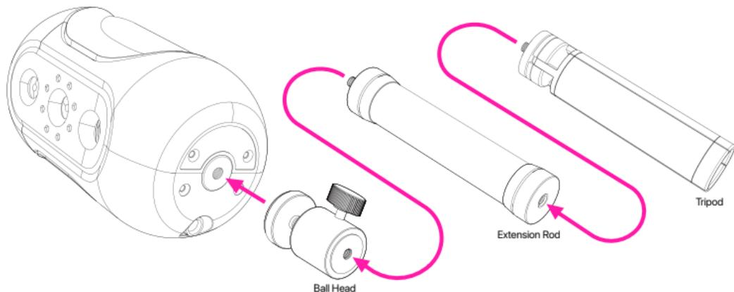
Connect the tripod to the extension rod by inserting the screw thread on the top into the screw hole in the another and tighten it clockwise;
